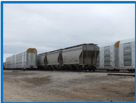
Auto Carrier Rack Cars with C4 Covered Hoppers (middle) at San Angelo TXPF Classification Yard, January 2020
